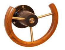
Model: WHZ. Follow up wheel. Mech. Travel ±90 EMRI teak wood Helmsman wheel. Stainless Steel Spokes. Seawater resistant aluminum. Black Anodized Chrome sealed. Diameter: 280 mm.
